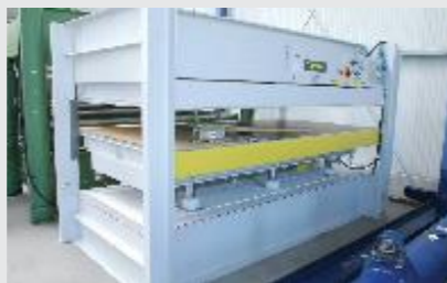
Veneering press used at veneering stage
