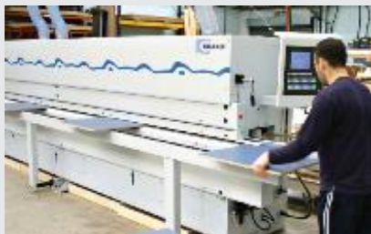
Edge branding machine used at veneering stage
